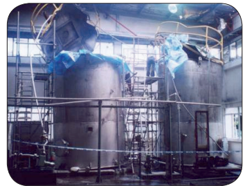
Figure 31: Exploded chemical storage tank.
