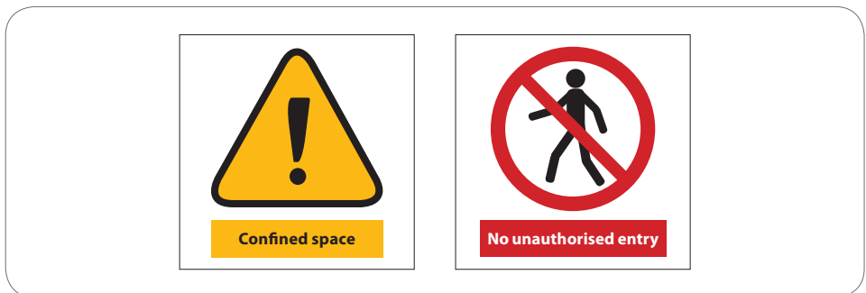
Figure 4: Examples of Confined Space warning signs.
