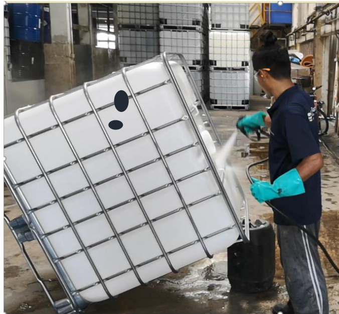
Cleaning the inside of an IBC using a water gun.
